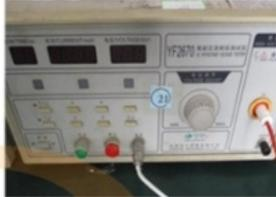
A white AC withstand voltage tester with a digital display and various control knobs and buttons. |
